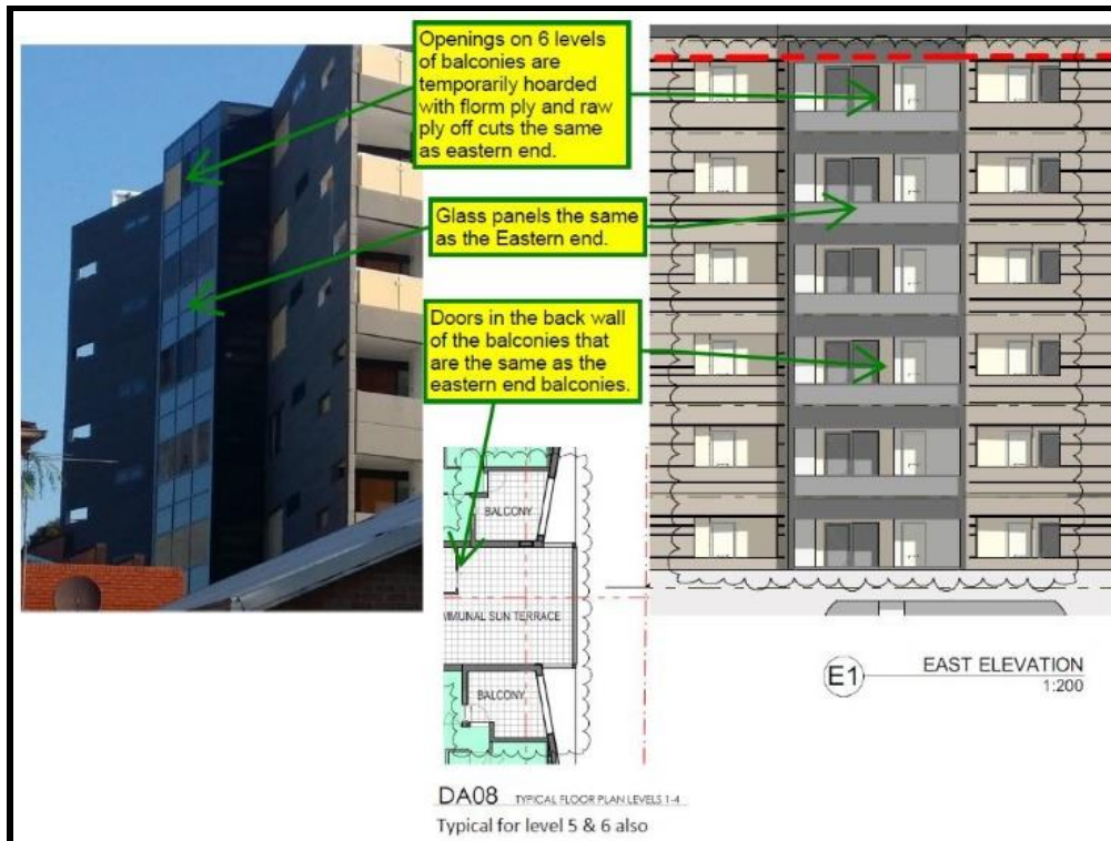
Figure 26: Applicant's explanation for works as completed and approved plans (Eastern elevation – Levels 1-6)
